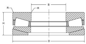
T-Flat Self Aligning Thrust Bearings
